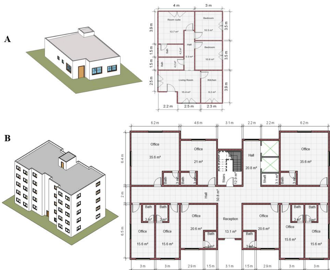
Figure 4.5 - 3D view and floor plan of A) residential building; and B) commercial building
