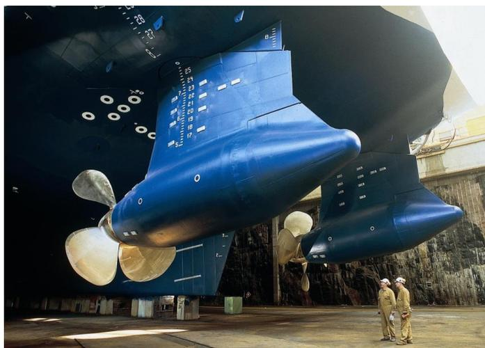
Figura 3.13 - Propulsor azimuthal
