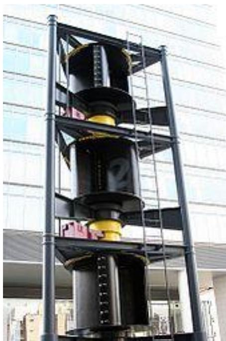
Figura 3.6 – Turbina Savonius [12]
